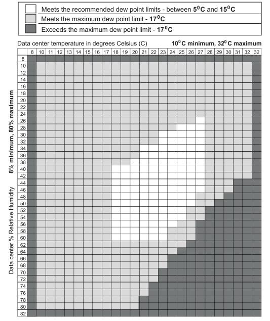
It is very important the environmental specifications be met immediately in front of the frame of the z10 server. Ideally, it would be best if the temperature and humidity controls are good enough to surround the service area of the z10. If you are able to exceed the required conditions, focus your efforts to provide the best guality air at the bottom front of the server.
