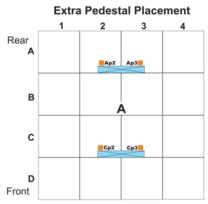
All pedestals should be adjusted to just contact the underside of each floor panel **before** the frames are rolled into place. Depending on your floor panel type, additional supports (pedestals) may be necessary to restore the structural integrity of cut panels.
