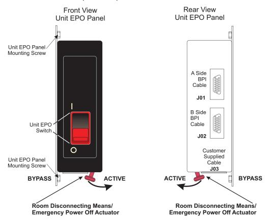
This figure illustrates the back of the machine UEPO panel showing where the room electrical power disconnecting means, or room Emergency Power Off, EPO, cable plugs into the machine. Notice the switch actuator. Once moved to make the cable connection possible, the room disconnecting means / EPO cable must be installed for the machine to power on.
