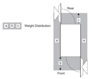
Floor loading for servers without Internal Battery Feature
