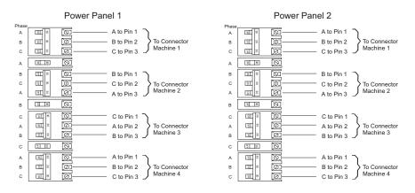
Figure 3. Power load balancing - alternating three-pole and single-pole breakers
