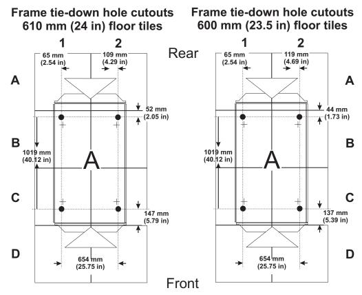
Additional floor panel pedestals may be necessary to restore structural integrity to the raised floor after making the circular cuts for the turnbuckles. Consult your flooring manufacturer for recommendations.
