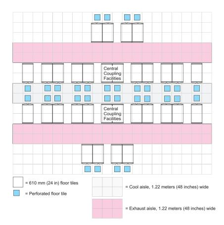
By following these guidelines, you will be able to configure a Parallel Sysplex, using the minimum amount of floor space, that meets your performance and availability objectives. The use of technology combinations - z10 EC, z10 BC, System z9, zSeries, and S/390 servers and coupling facilities - may complicate your physical planning, but the basic strategies outlined here will result in a successful Parallel Sysplex environment.
