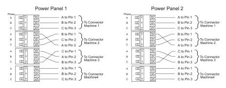
Figure 2. Power load balancing - three-pole breakers
