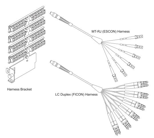
There can be from one to five rows of trunk connectors on the bracket. The trunk brackets use an MTP connector, and the FICON and ESCON connectors are routed to the feature cards in each frame.
