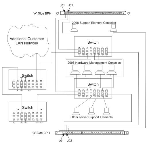
The following illustration provides general z10 BC Ethernet cabling information and is not intended to illustrate connection to a particular network.
