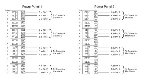
Figure 4. Power load balancing - alternating three-pole and double-pole breakers
