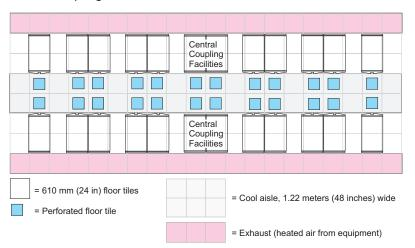
5. As the Parallel Sysplex evolves, you may eventually exceed the 7 meter usable length of ICB cables at the ends of a two-row configuration. At this point, it may be possible to add rows, using ISC links or InfiniBand links, which provide connectivity over greater distances than ICB links. With the equipment in these new rows centered on the original central coupling facilities, the Parallel Sysplex now assumes the shape of a diamond.
