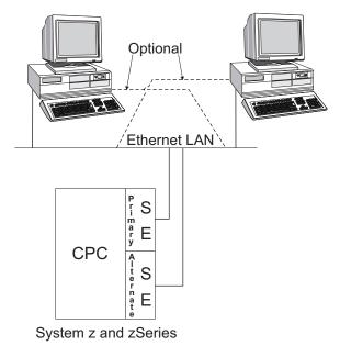
Additional connections to the Ethernet LAN may be made to expand the connectivity beyond the local Hardware Management Console and Support Element.
