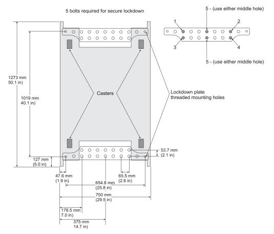
The stabilizer fasteners should be heavy duty sleeve anchors, 12 mm (0.5 in) in diameter, capable of withstanding a minimum allowable tensile load in concrete of 1025.1 kg (2260 lb) and a minimum allowable shear load in concrete of 2111.5 kg (4655 lb). The contractor you engage to install the stabilizers will determine the length of the anchors.
