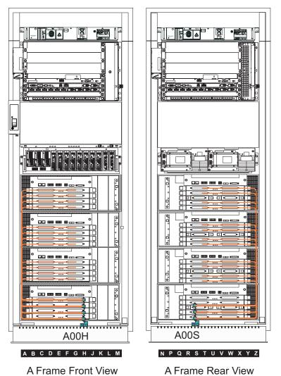
This illustration shows the Fiber Quick Connect bracket features at A00H in the front of the frame and A00S in the rear.
